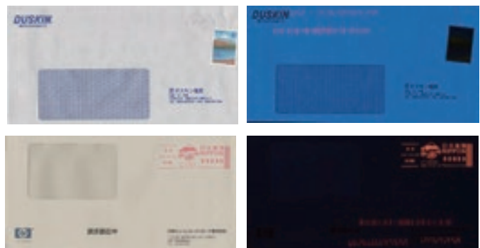
Mail barcode printed with fluorescent ink Visible light image ( left ) / fluorescent light image ( right )
